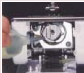
Oiling the rotary hook system
