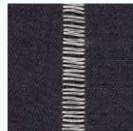
Serged flatlock seam after being pulled flat.
