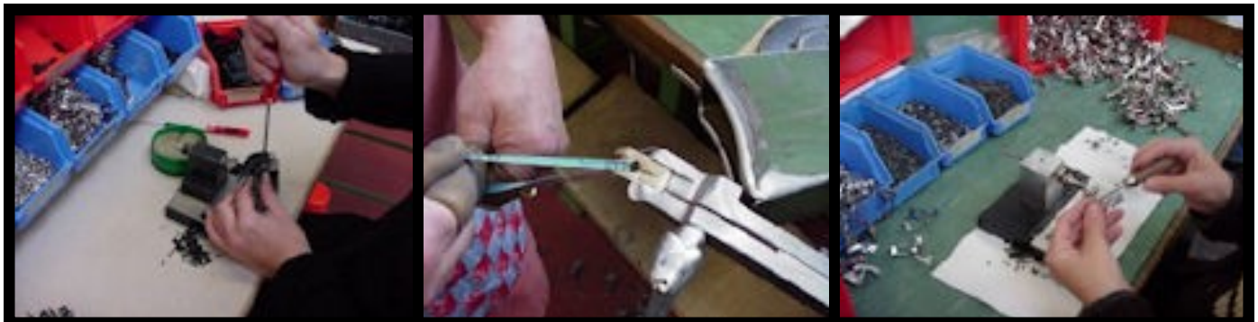
Assembling the Walking Foot • Hand-polishing Presser Feet Soles • Assembling the Blind Hem Foot
