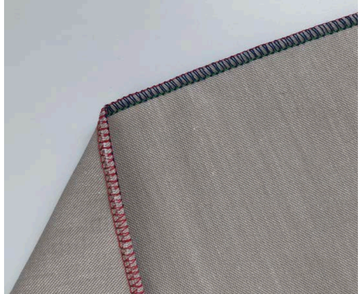
The 3-thread narrow seam creates a nice secure seam for fine fabric
