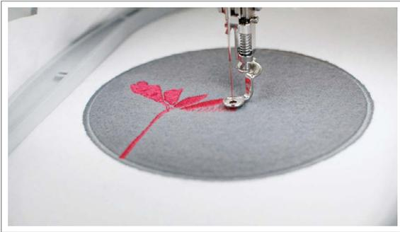
Ensure that the needle is free of burrs and is not dull or bent.
