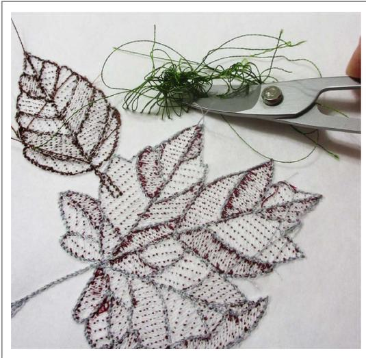
**NOTE:** Stop the machine and cut away the thread nest as soon as it occurs so that the threads don't become trapped as the design continues to stitch.
