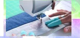
The vertical spring action presses the foot to the fabric, preventing the fabric from lifting along with the needle, and therefore ensuring perfect stitch formation.
