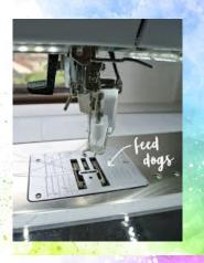
Free motion quilting is quilting using your domestic sewing machine without the aid of the feed dog of the machine or a long/mid arm machine on a quilt frame.
