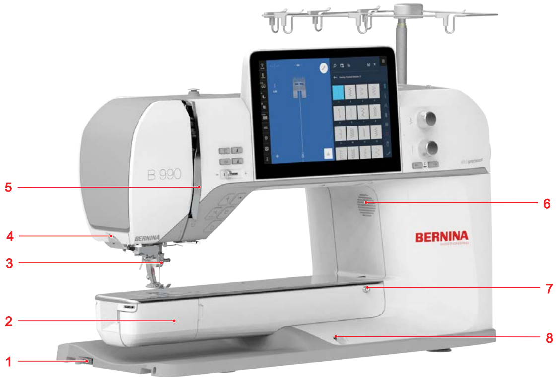
1 Embroidery Module Connection 2 Bobbin Cover 3 Needle Area 4 Thread Cutter 5 Thread Take-up Lever Cover 6 Speaker 7 Connection for Slide-on Table 8 Knee Lifter Connection
