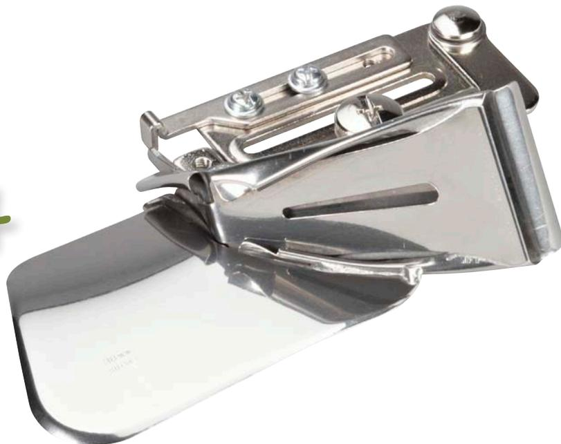
Available in three sizes, BERNINA Binder Attachment #88 holds, folds, and wraps a fabric strip around a project edge, completely enclosing and finishing it. This attachment secures to the bed of the sewing machine with a single thumb screw and requires the use of Binder Foot #95/95C, sold separately. This useful attachment provides a speedy professional finish to the edges of quilts, garments, craft projects, and home decorating items.
