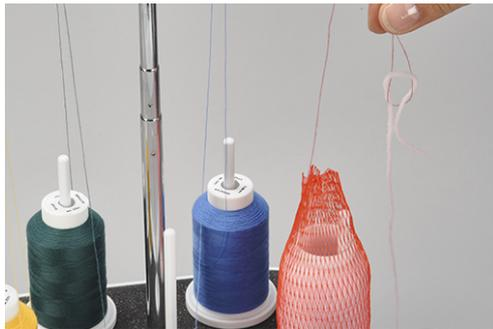
> Pull the threaded end of the thread until the newly knotted thread is in front of the needle eye.
