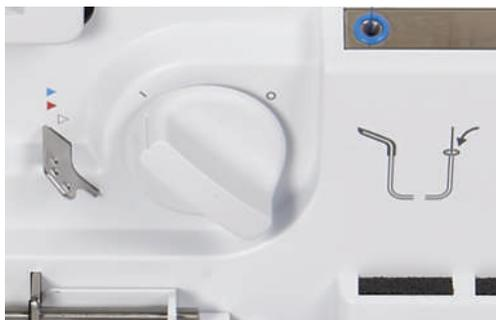
> Turn the air threader connection completely in the required direction.
