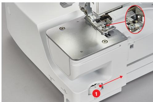
– The knife, the stitch finger and the looper cover move in the corresponding direction as a result of the set knife position.
